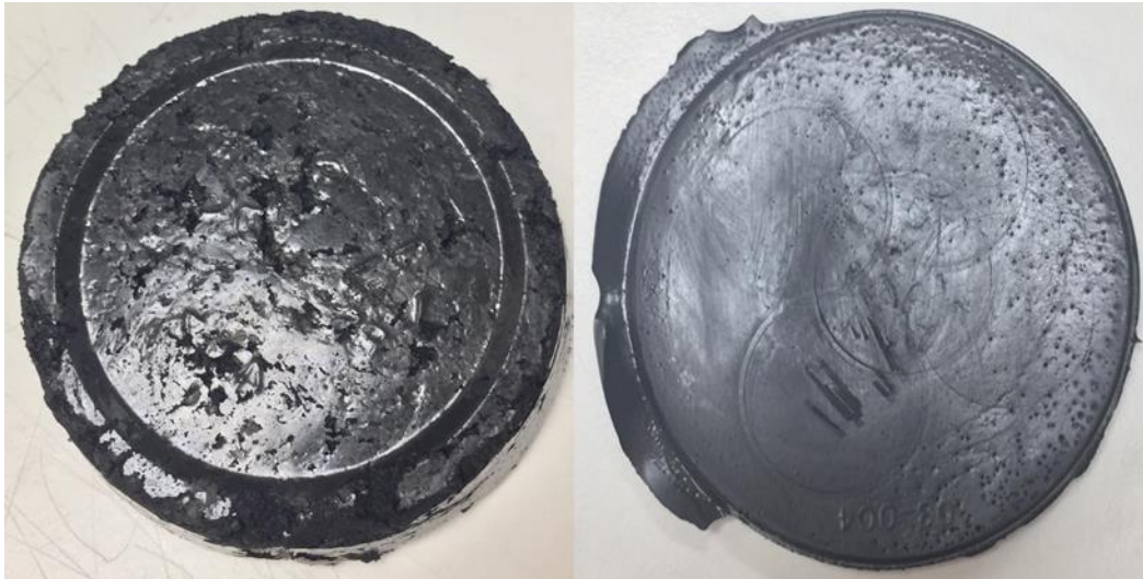
Figure 4.2 Comparison of cured samples from old recipe sample [82, 83] (left) to new recipe sample (right). Surface finish of the new sample is finer and has fewer cracks than the old recipe.
